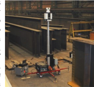
The Bridge Virtual Assembly System's laser detection allows bridge girders to be fitted via a computer model rather than manually in fabrication shops.
